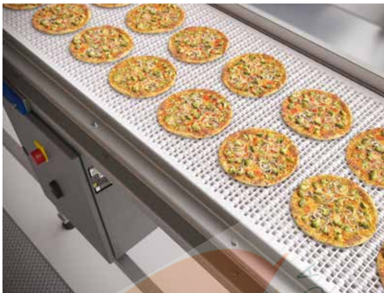
Conveyor equipped with Rexnord 1096 Series KleanTop Belt.
