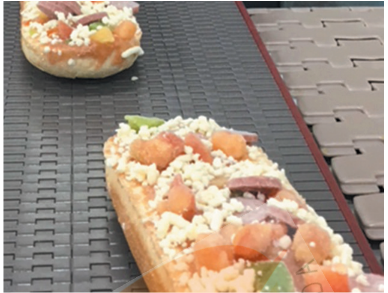
Conveyor equipped with Rexnord 395 Series KleanTop Belt.
