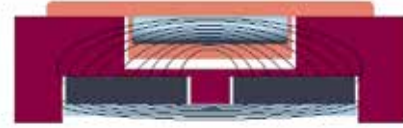
Magnetflex® curve with 2 magnets for better hold-down of the chain
