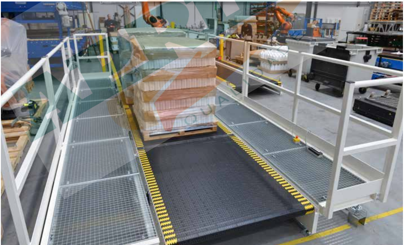
Conveyor equipped with Rexnord 1020 Series MatTop Chain
