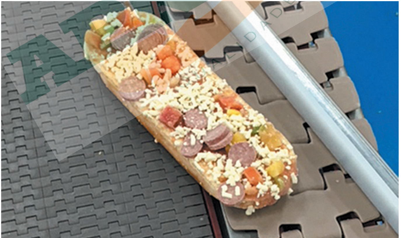
Conveyor equipped with Rexnord 395 Series KleanTop Belt.
