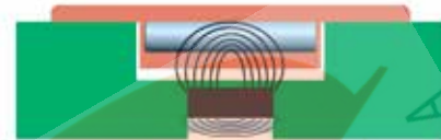
Usual magnetic curve with only 1 magnet
