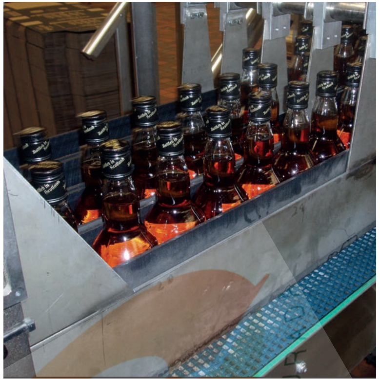
Conveyor with 500 belt.
